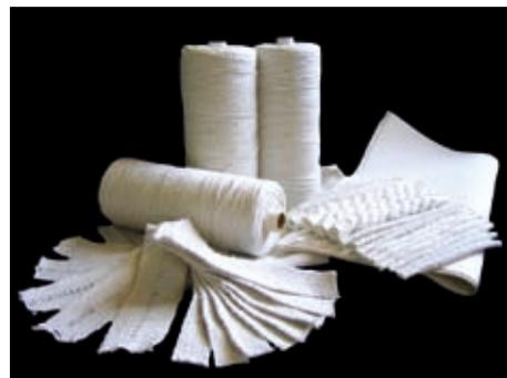
CMAx ceramic fiber textiles contain carrier fiber to facilitate the carding process. The textiles normally contain 16-20% rayon fiber which will burn out at high temperature, but has no effect on the properties of the products.
